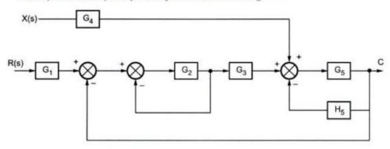
Solution: With X(s) = 0, block diagram reduces as,
