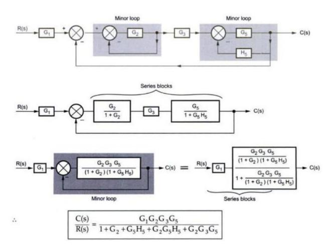
With R(s) = 0,  $G_1$  vanishes but minus sign at summing point must be considered by introducing block of -1, as shown.
