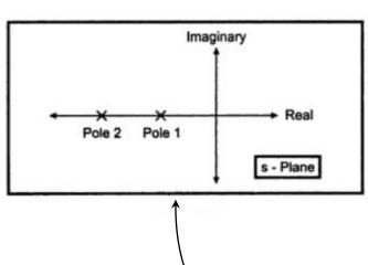
So system is 2nd order and the two poles are,  $-\frac{R}{2L} \pm \sqrt{\left(\frac{R}{2L}\right)^2 - \left(\frac{1}{\sqrt{LC}}\right)^2}$
