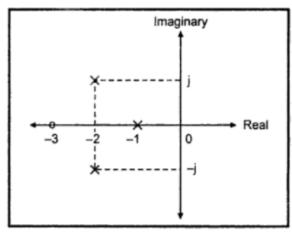
Sol.: From pole-zero plot given the transfer function has 3 poles at s=0, s=-1, -2+j and -2-j. And it has one zero at s=-3.
