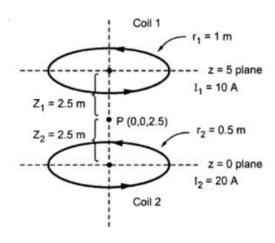
Assuming direction of  $I_1$  and  $I_2$  same, according to right hand rule  $\overline{H}_1$  and  $\overline{H}_2$  at P due to coil 1 and coil 2 are in same direction i.e.  $\overline{a}_z$  direction.
